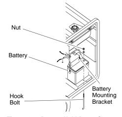
Figure 10 - Battery Hold-Down System (Model PGH11000IE Shown)
